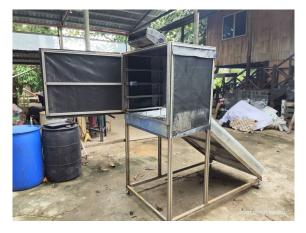
The prototype adopted from design learnt from SIBAT, Philippines. Used lightweight materials such as Geomembrane and UV Plastics. It also has capability to be connected to ballast load of solar hydro system to utilise excess energy from RE system. Can also be used using electricity (1 kw) should need to operate at night. Thermal insulation improves the heat retention.
